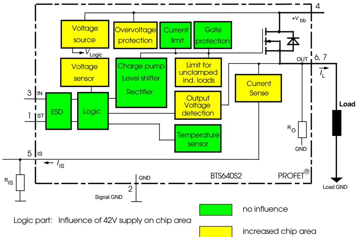
Fig. 4: Effect of higher supply voltage on the integral logic part of a smart power switch such as the Sense PROFET BTS640S2
