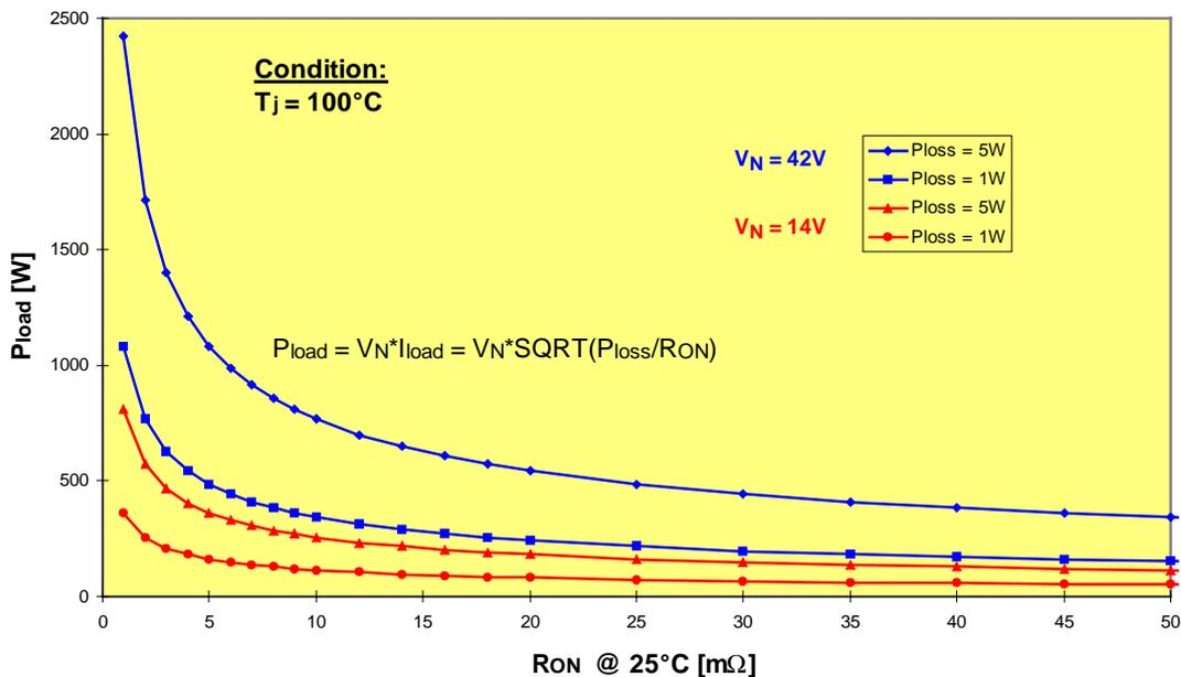
Fig. 5: Switchable continuous load as a function of on-state resistance for 14 V and 42 V power supplies
