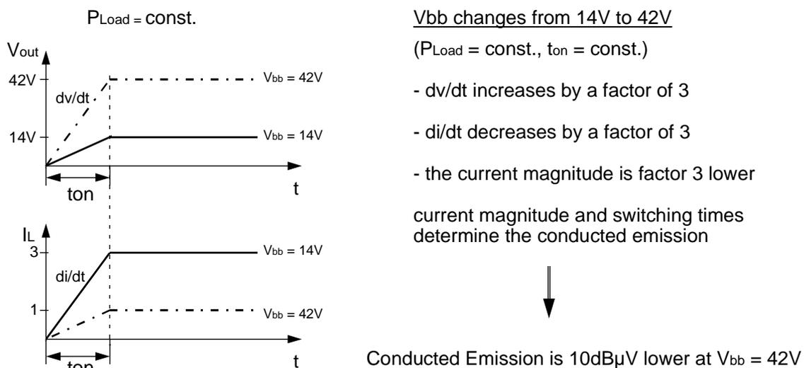
Fig. 8: Illustration of turn-on slopes for voltage and current achieving the same turn-on time with a 42 V or with a 14 V supply
