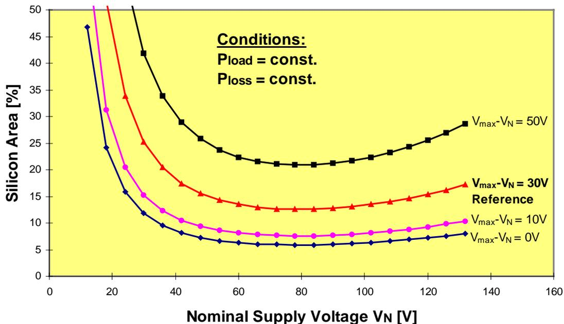
Fig. 3: Effect of the additional required withstand voltage  $V_{add}$  on the resulting power chip area as a function of the nominal supply voltage
