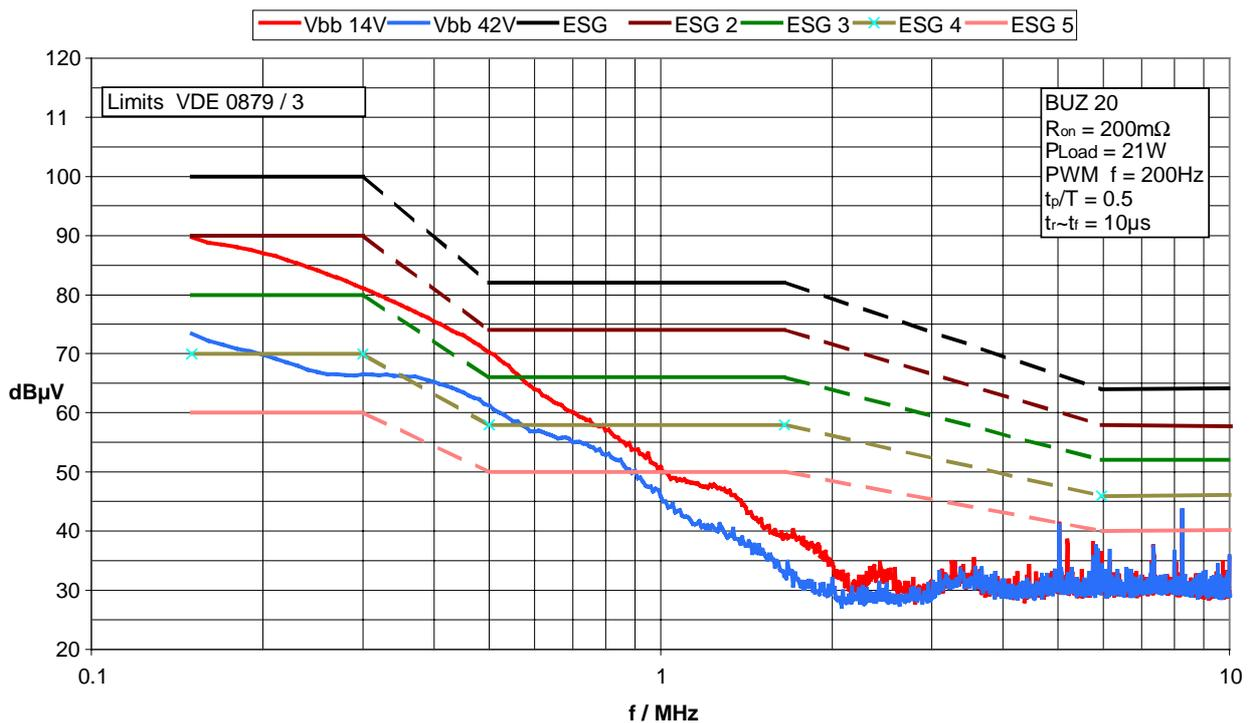
Fig. 9: Different spectra of conducted electromagnetic emission on the positive supply voltage conductor at 14 V and at 42 V supply and 200 Hz PWM frequency
