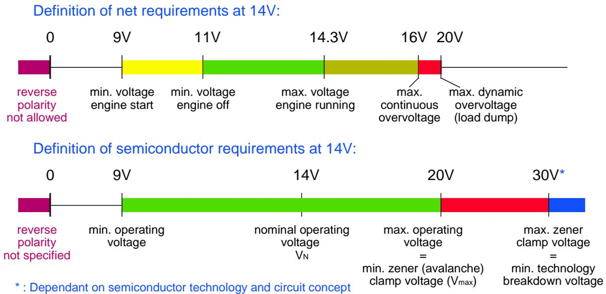
Fig. 7: Voltage definition of future power switches for the 14 V system
