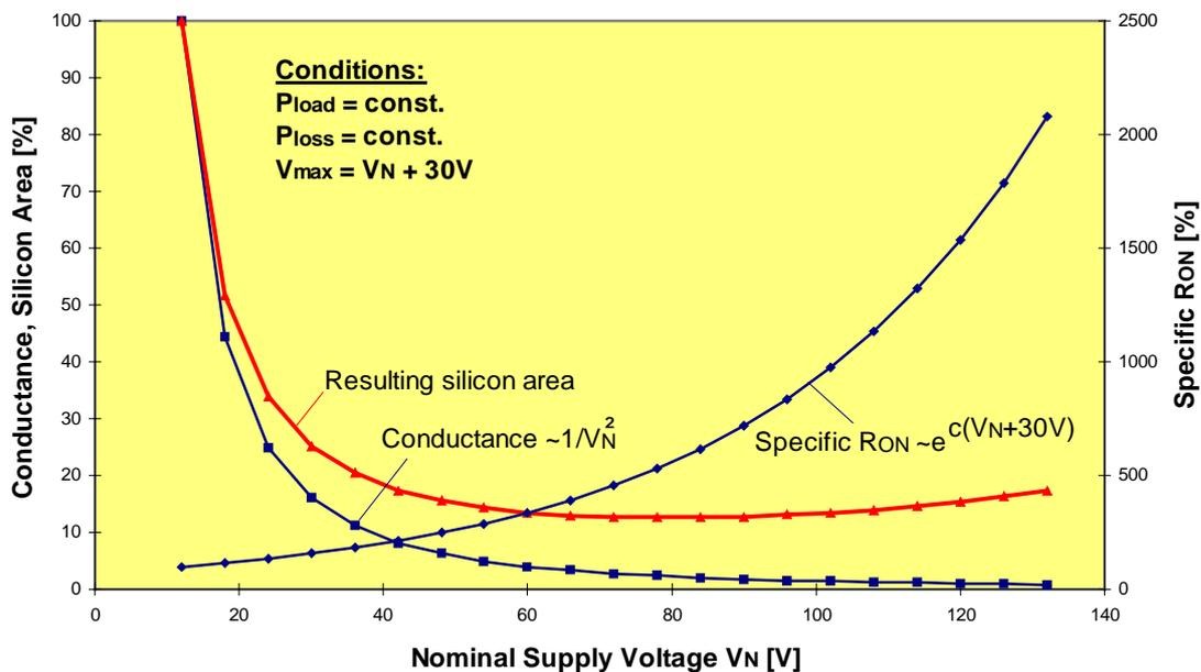
Fig. 2: Necessary silicon area for the vertical power semiconductor switch as a function of nominal supply voltage
