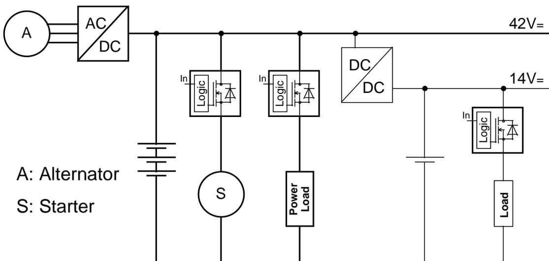
Fig. 1: Simplified automotive electrical system for the future with 14 V and 42 V dc supply
