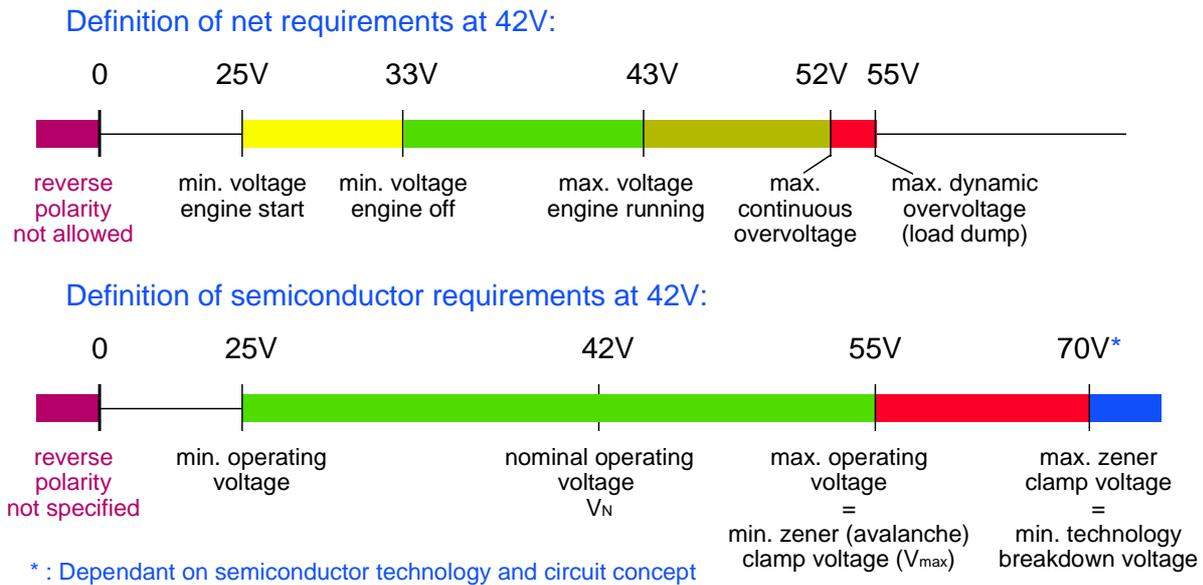
Fig. 6: Voltage definition of future power switches for the 42 V system
